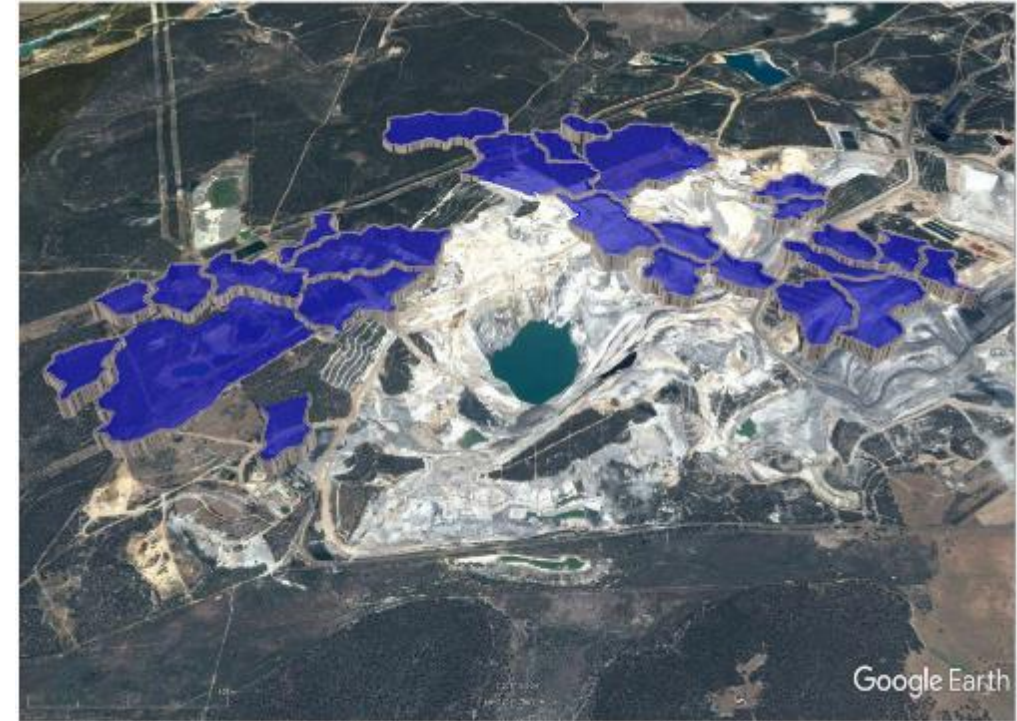
Figure 15: Potential PHES upper reservoir sites at Collie, WA, with 200 m head into the pit and a good volume of stored water.
